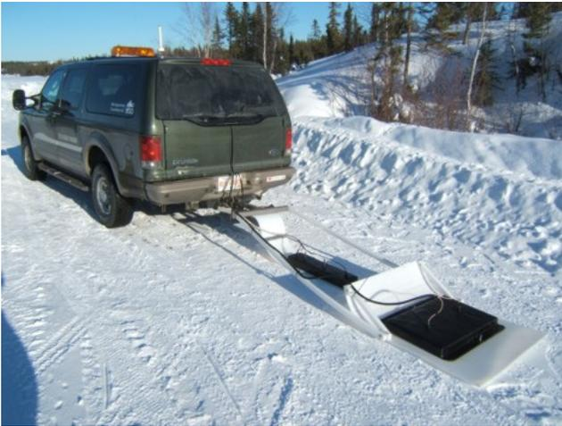
Figure 7. Dual channel ice radar system for combined ice thickness and water depth.
