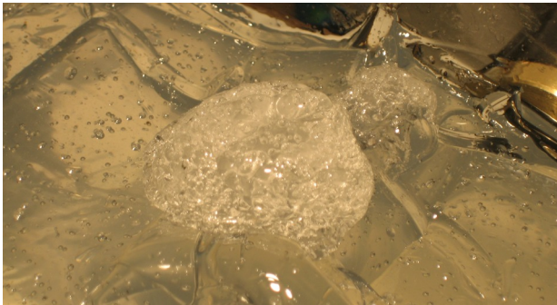
Figure 14: Large cone in foreground with smaller cone in rear on top of gas escape structures
