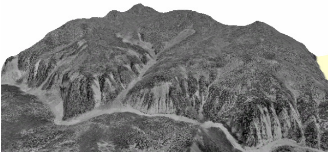
Figure 5. Large low-gradient landslides and smaller, steeper, closely spaced ones on the south slopes of Buckingham River. The 1730 m long retrogressive landslide (centre) occupies a buried valley and has a travel angle of 6.7^\circ . The steeper smaller landslides typically have 17 or 18^\circ travel angles.
