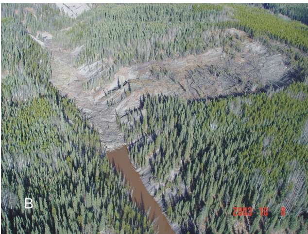
Figure 4. Contrasting flows in the Buckingham area. The very wet flow in (a) travelled 600 m at 12.5^\circ . Because the landslide entered a large river, its dam was short-lived. (b) a 700 m flow in with a travel angle of 8.5^\circ impounded a small tributary of Buckingham River. The dam has remained in place for approximately a decade.
