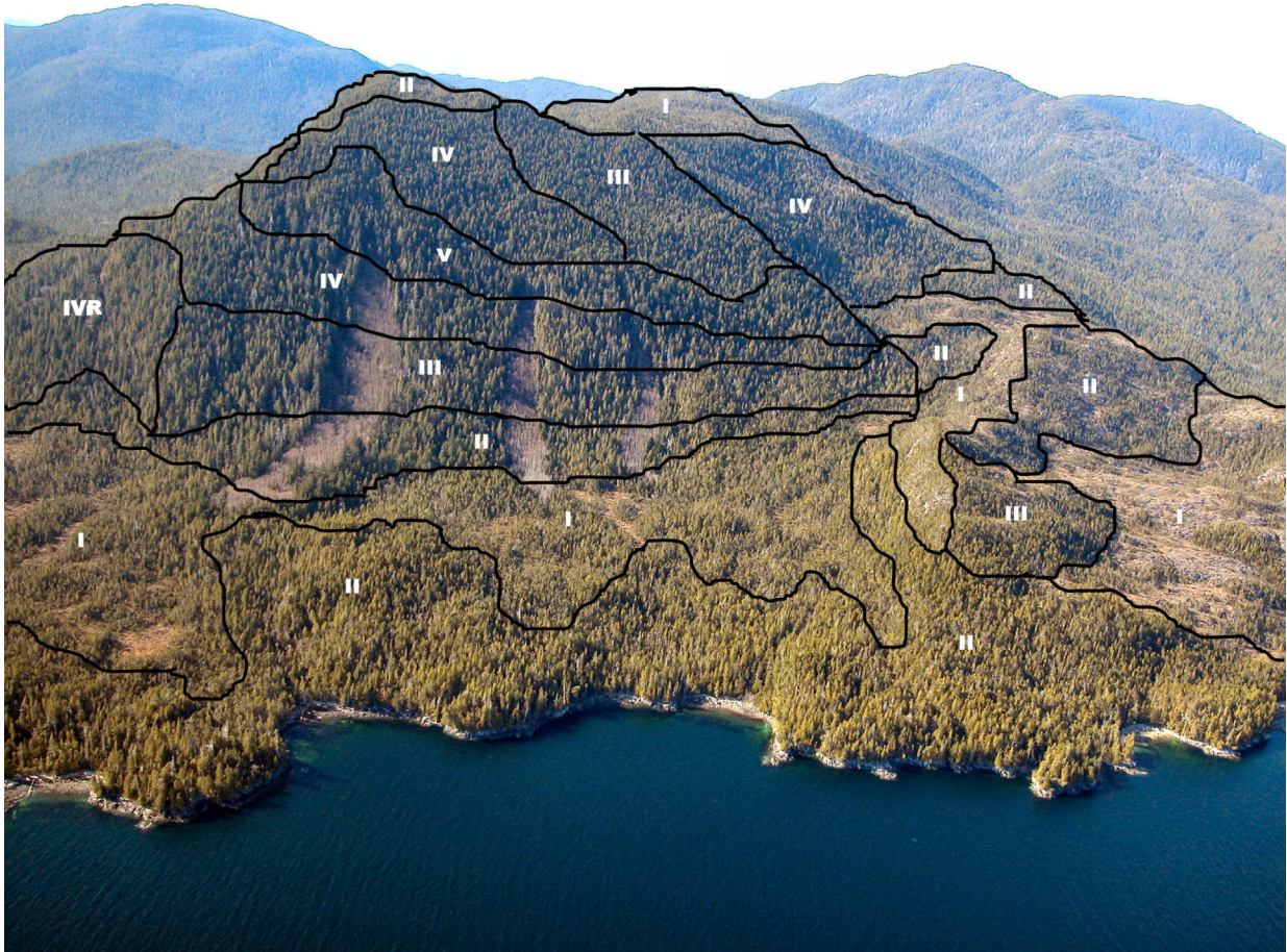
Figure 6. Example polygons of five class terrain stability mapping. Projection is onto a landscape on the BC north coast. Classification is presented in Table 3.
