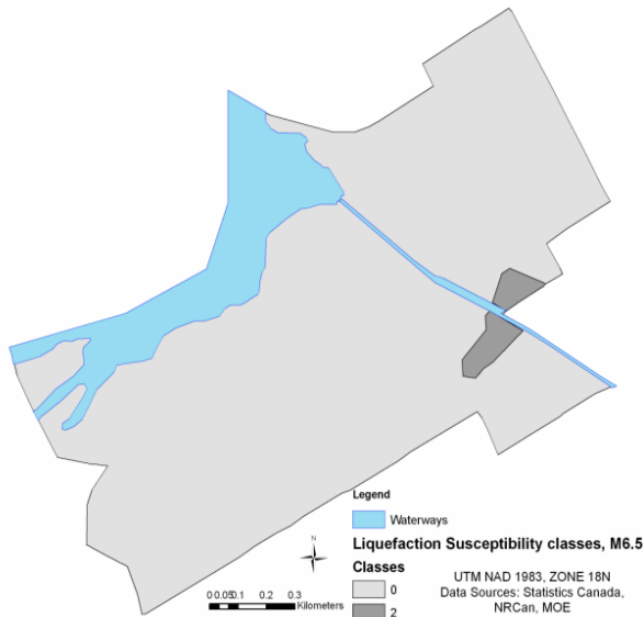
Figure 4. Probability of liquefaction map for M_w6.5 scenario. (Data sources: NRCan, MOE, Stats Canada)
