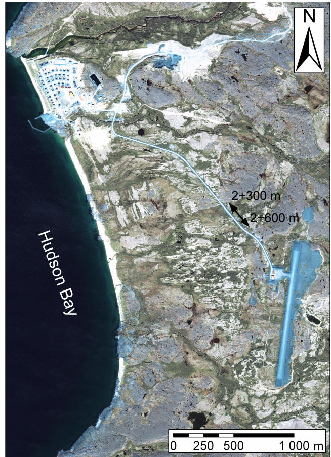
Figure 3: Inuit community of Umiujaq. The ends of the 300-meter long road segment affected by thaw subsidence are identified according to the location system of the Ministère des Transports du Québec (1991).
