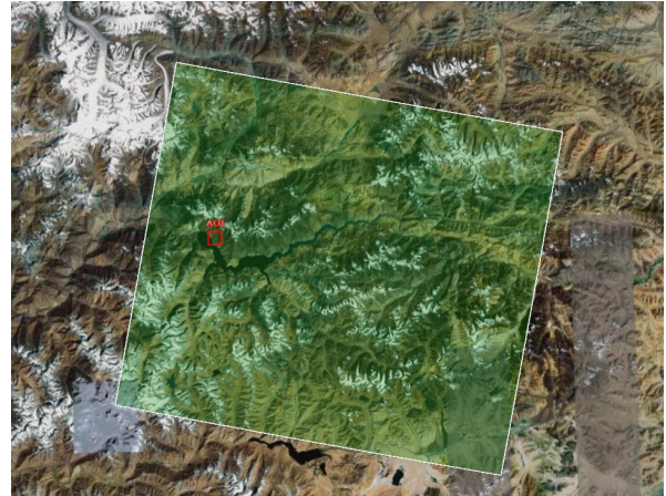
Figure 9: Relative position of the Envisat Track 5 - Frame 2837 Descending orbit. Lake Sarez RBS is indicated in the small square.
