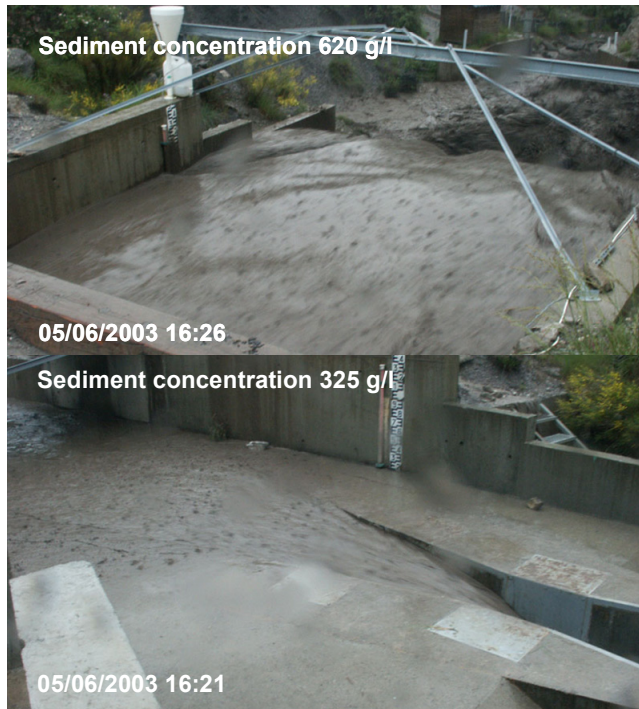
Figure 5: Highly concentrated flow in the Laval station
